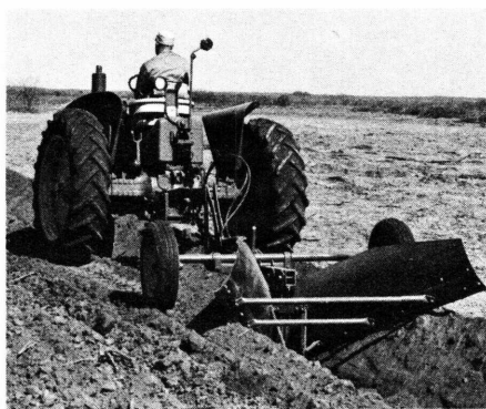
Figure 1.—This implement is a type used to open furrows for setting asparagus crowns. The blade can be adjusted to make furrows of the proper depth.
